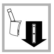
**5.** After the timer expires, wipe the vial and insert it into the cell holder.
