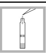
**2.** Pipet 0.5 mL of sample into the vial.
