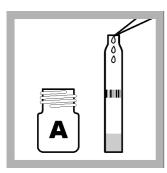
1. Pipet 2.0 mL of **Solution A** into the test vial.
